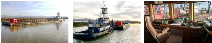
Specifications : VESSEL NAME: Seana C DIMENSIONS: 70' x 24' x 7.5' BUILT: 1975 CLASS: Sub-M Certified MAIN ENGINES: (3) QSK-19 HORSEPOWER: 1980 @1,800RPM TIER RATING: 3 REDUCTION GEARS: (3) Twin Disc MG 527 5.17:1 GENERATOR: (2) Marathon CAPACITY: (2) 65 KW
